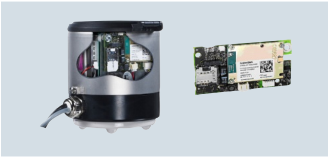
GSM/GPRS communication module
